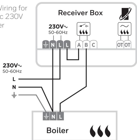
**B)** Wiring for Combi boiler
