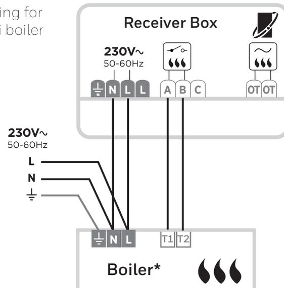
**C)** Wiring for OpenTherm boiler
